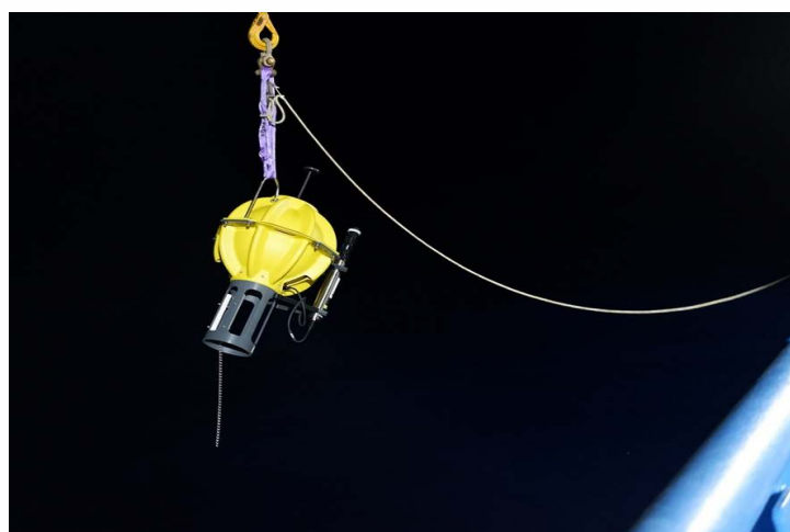
Figure-3: The spherical Deep Argo float being deployed by crane into the Indian Ocean before dawn from the RV Investigator (Photo: Karlie McDonald)
