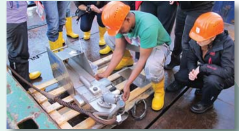
A Continuous Plankton Recorder is being prepared for deployment. Photo Credit: Alfred Wegener Institute / Philipp Wenta.
