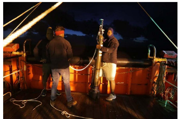
Deployment of ARGO float with CTD, oxygen, nitrate, FLBB bio-optical and pH sensors
